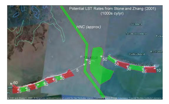
Figure 13. Application of net longshore transport rates from Stone and Zhang (2001) into a calculated sediment budget for sand transport under non-storm conditions
